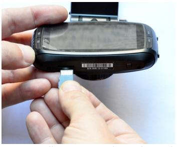
Install microSD Card into the card slot.
