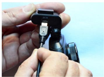
4. Connect Power cord to the DC IN Camera power socket.
