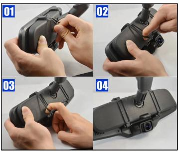
1. Use the clips on the back of the CM PRO to mount it onto your rear view mirror.
