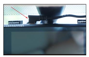
4. Connect Power cord to the DC IN Camera power socket.
