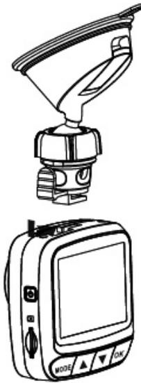
2. Attach the bracket to the camera. Slide it into the bracket holder until you hear a click.
