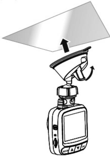
3. Remove the protection tape from the Suction Cup and onto windshield. (We recommend to clean the installation area with rubbing alcohol). Then securely lock it. Usually the best result is when the camera is installed near the top of the windshield behind the rearview mirror. The camera lens has to be closest to the glass for prevent reflection.
